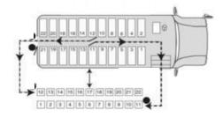
If the bus is on the side, use the roof hatches as well as the emergency doors on the up side to evacuate students. The windshield and rear windows can also be pushed out to facilitate evacuation.
